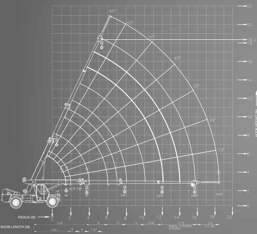
Rate loads are calculated for operation on leveled surface.
